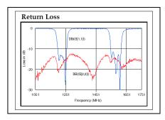
As can be observed, the use of dual diplexed filters (either L1/L2 or L1/L5) results in symmetrical passband characteristics.
