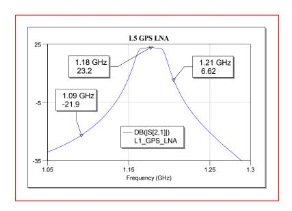
A 3-pole ceramic filter attenuates the transmitted RF pulse by 44 dB, reducing it to a level that is tolerable to a companion GPS receiver.
