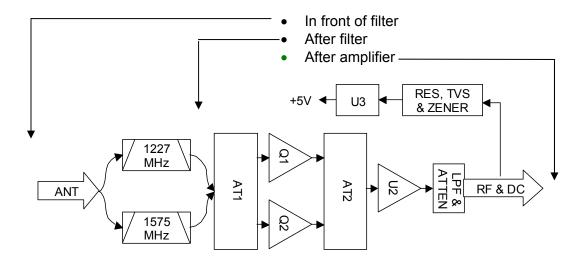
The limiter diode acts as a non-linear circuit element when pulsed resulting in the generation of numerous spurious products. This position provides the most frontend protection, but at the expense of reduced anti-jam operation. Another disadvantage to this placement choice is that the limiter acts upon all signals, even those outside of the filters' passbands.
